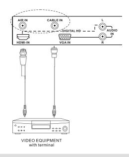
Note: If you have an off-air antenna or cable TV, connect the off-air antenna or TV cable to the RF connector on the rear of your VCR.
